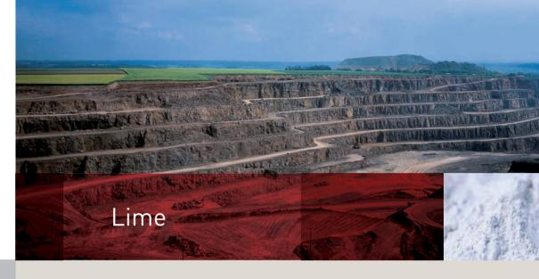
Air lime is produced by heating high pure limestone at temperatures around 900°C.
